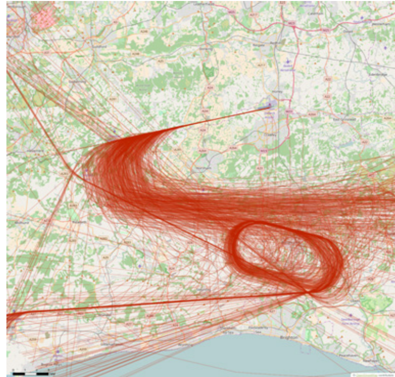
Figure 17: 24 Hour Period Of Easterly Operations (Runway 08R) Showing Arrivals Only - Map 1 of 2
